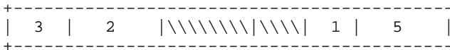
Figure 6.10. The codebook memory, length lMem=147 samples, and the target vector 5, length 40 samples
