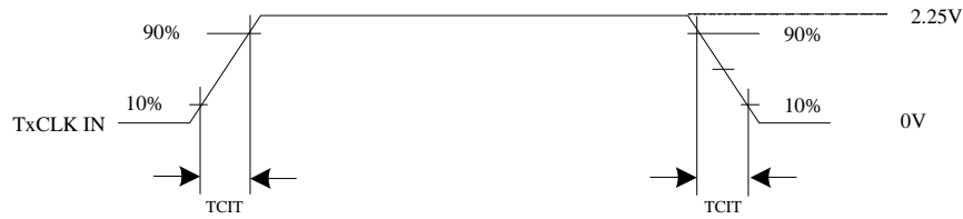
Figure 5. Tx Input Clock Transition Time
