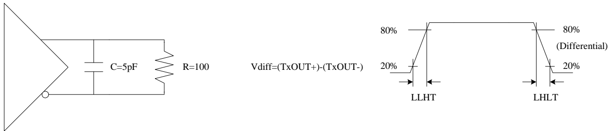
Figure 6. LVDS Output Load and Transition Time
